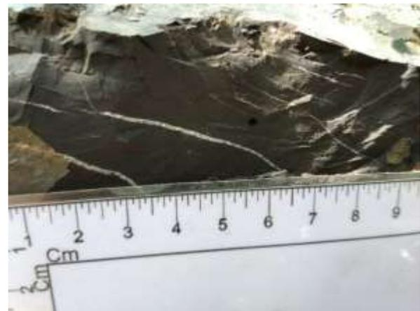
Figure 11. Quartz vein on silicified coal.
