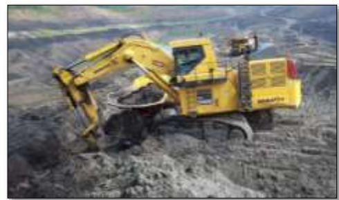
Gambar 4.2 Excavator Komatsu PC 2000
